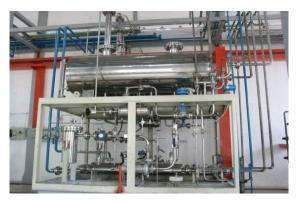
DM Water is continuously supplied by a Feed water pump which operates at the operating pressure of the system. This DM Water is used to generate the Hydrogen and is consumed @ about One liter per Nm3 of Hydrogen Generated.
